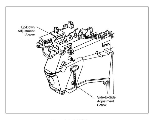
Figure 3-5 Grid Adjustments
